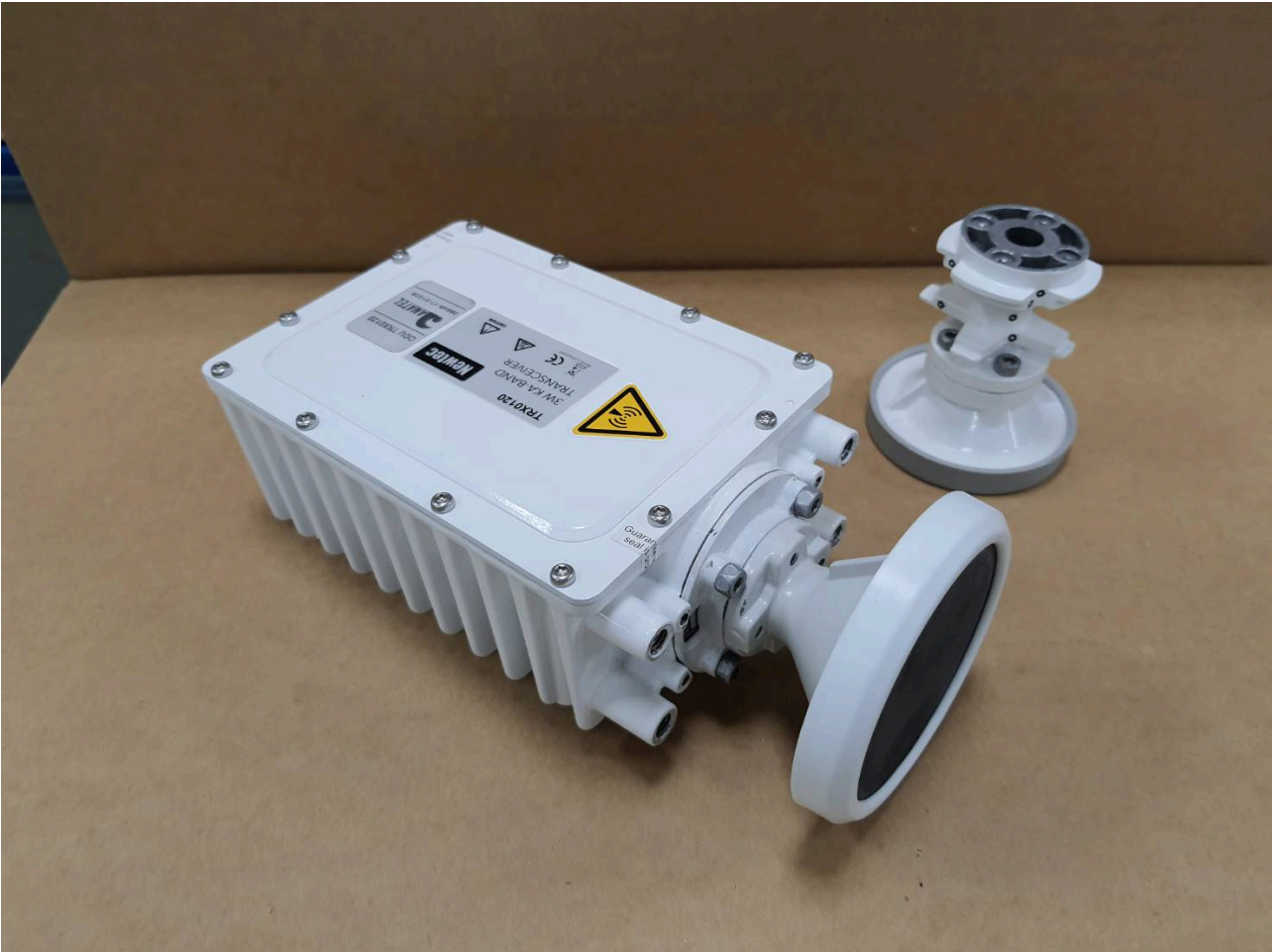
Re-assembly with new feedhorn without the waveguide, note the polarization according to beam table
